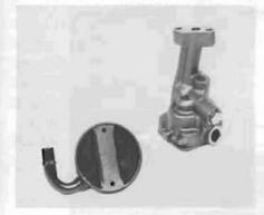
A high-volume, high-pressure oil pump can be a real engine saver. This stock-configuration pump requires no changes or modifications but provides idle pressure readings of 45 lbs., and pins the needle at 80 lbs. in a motor with a good bottom end. A must if you're rebuilding your motor or going autocrossing; recommended for all cars that are driven hard.
