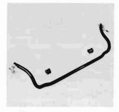
The final step for the chassis tuner is an adjustable anti-sway bar. Heim joints provide instantaneous bar-to-chassis reaction and preloading of the suspension. The sway bar can be used to compensate for imbalances (such as a car that handles better in left-hand turns than right-hand turns) in handling, or to tune the chassis to the driver's preference of oversteer, understeer, or neutral handling characteristics.
