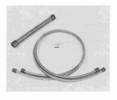
One of the most eye-catching additions to an engine compartment is braided steel radiator and heater hose. It looks great while eliminating those breakdowns that always happen at the wrong time.
