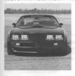
Originally a very limited production item, this fiberglass nose piece is now being offered to all Trans Am enthusiasts. The nose was specifically designed to alleviate the Trans Am's borderline engine cooling, and has proven itself capable of flowing enough air to keep even a heavily-modified big-block running at satisfactory temperatures.
