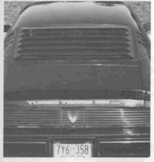
Add a sophisticated sporty look to your car with wrap-around louvers for your backwindow. These 3-piece louvers feature aircraft-quality aluminum and stainless steel construction with a hinged center section for easy cleaning. By blocking sunlight, they reduce the load on the air conditioner and protect the car's interior from fading, yet do not obscure vision. Flat black finish matches every car.
