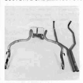
We've designed a dual exhaust system which incorporates two front pipes, two mufflers (which fit snuggly in the cavity under the rear seat) and two tail pipes with chrome splitters. This system is very free-flowing and makes the car sound like it should have sounded from the factory — while still retaining a very respectable tone. This system is worth gains of 25 horsepower and 2-3 mpg. Excellent as a first modification, and even better in conjunction with headers.
