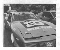
The same fiberglass fenders used on our Daytona entry. These fenders weigh only 13 lbs. each, to cut front end weight, yet are strong enough to hold up at over 200 mph. They provide clearance for any tire you can fit on an eleven inch wheel for racing or for outrageous street looks. Front fenders are bolt-on, but require modification if used with our air dam. Rear quarters must be bonded or riveted on.
