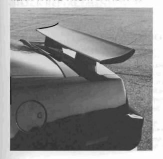
The counterpart to our front air dam is this very aggressive rear wing. Like the front wing, this piece is effective from highway speeds on up to over 180 mph, producing the downforce needed for high-speed cruising/racing stability. Gives your car an unmistakable look.
