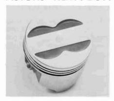
At Trans Am Specialties, we use only forged pistons in our engine buildups, and we offer only these pistons to our customers. They are stock configuration, but provide far greater durability and reliability than any cast piston.
