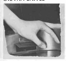
If you take advantage of your Trans Am's superior cornering ability, you may have noticed that in tight cornering situations, oil pressure takes a big drop. Even a stock Trans Am can suffer oil-related engine failure under sustained hard cornering, as some unfortunate owners have found. Our oil pan baffle solves 99% of these oiling problems. The baffle kit requires minor welding. Can be installed in about 3 hours. For stock 400-455 oil pans with windage trays (covers 90% of all Trans Ams).
