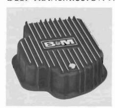
The simplest way to protect your automatic transmission from high temperatures is with a deep pan. These pans provide 3-4 additional quarts of fluid capacity. Choose chrome-plated steel for light weight, low cost, and good looks, or black cast aluminum for additional heat dissipation, superior transmission rigidity, and good looks.
