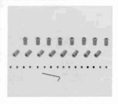
Under high rpm conditions, stock rocker arm nuts can back out of adjustment. Poly locks have a special double-locking action to ensure that valve lash stays put, eliminating unwanted valve train movement and possible damage. These poly locks are made of high-strength steel, and will not fail under high-rpm loads.
