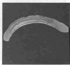
These fiberglass replacement inner wheelwells are used to provide tire clearance for sizes up to P245/60-15 or P245/50-15 for significantly better handling. Lightweight and easy to install.
