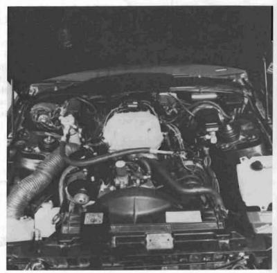
This engine produces 300 net hp @ 5500 rpm, with a redline of 7000. Performance: consistent 13.8 second ¼-miles (3.73 gears, street tires, through street exhausts) with a top speed of 150 mph. The car is very streetable, runs all power accessories and air conditioning, and requires only normal attention.
