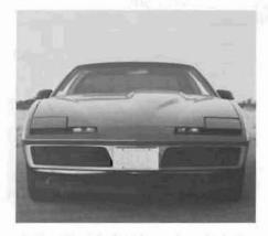
This nose can be used with either stock or Trans Am Specialties body parts to cut pounds from front end weight for a significant handling improvement. Also excellent for accident repair.
