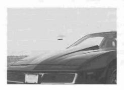
The centerpiece of weight reduction in our aero package is this fiber-glass hood. It cuts hood weight by about 50% for better handling. The sleek hood bulge is centered to provide clearance for high-rise manifolds, nitrous systems, or superchargers.
