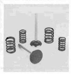
We use this combination in our motors for long valve train life and improved breathing. Both the intake and exhaust valves are of one-piece construction with hardened tips (no wear caps). The intakes are stock configuration and size (2.11"), while the exhausts are larger than stock (1.77" instead of 1.66") to improve the Pontiac's weaker exhaust side flow.
