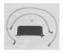
Just as heat is the primary enemy of your engine's motor oil, it is also the primary enemy of transmission fluid. A transmission cooler is good insurance against premature transmission failure on any automatic-equipped high-performance car; on a car modified for higher power output, a cooler should be a primary consideration.
