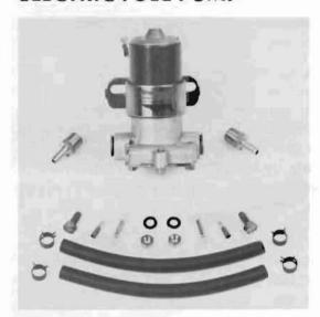
If your car requires higher fuel flow than even a high-volume mechanical fuel pump can provide (vapor lock problems, or dragracing use, for instance), then this pump is the answer. Designed to maintain a constant fuel line pressure of 5 psi (approx. 67 GPH), this pump assures adequate delivery for even multiple carburetor applications, yet does not require a regulator. Not recommended for fuel injection systems.
