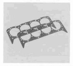
When it's time to do a top end engine rebuild, take the opportunity to add a bit more compression to your engine. These thin head gaskets raise the compression ratio about ¼ of a point, enough to raise a few more horses and improve throttle response without pushing you out of range of today's poor quality gasoline.
